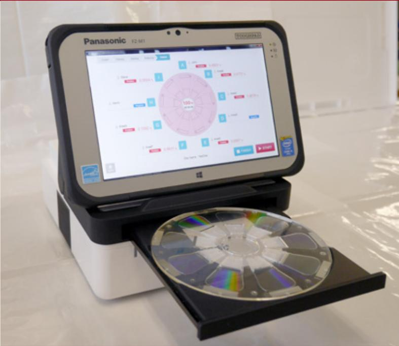
The portable, battery-powered device for malaria diagnosis developed jointly by AIST and a Japanese electrical manufacturer
