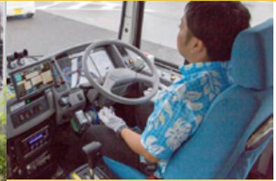
Test of an automated driving system using signals received from Quasi-Zenith Satellite System "Michibiki"
