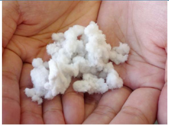
Used paper broken down into cotton-like fibers
