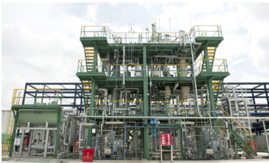
Reaction section in the SPERA Hydrogen® demonstration plant at Chiyoda's R&D Center in Yokohama Courtesy of Chiyoda Corporation
