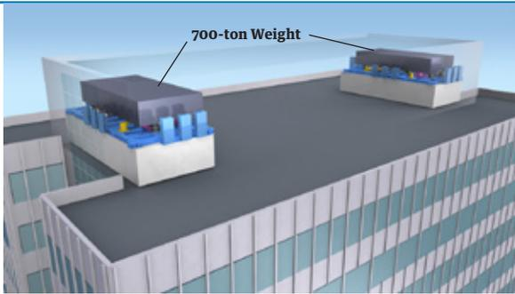
Image showing the two Dual TMD-NT vibration dampers
