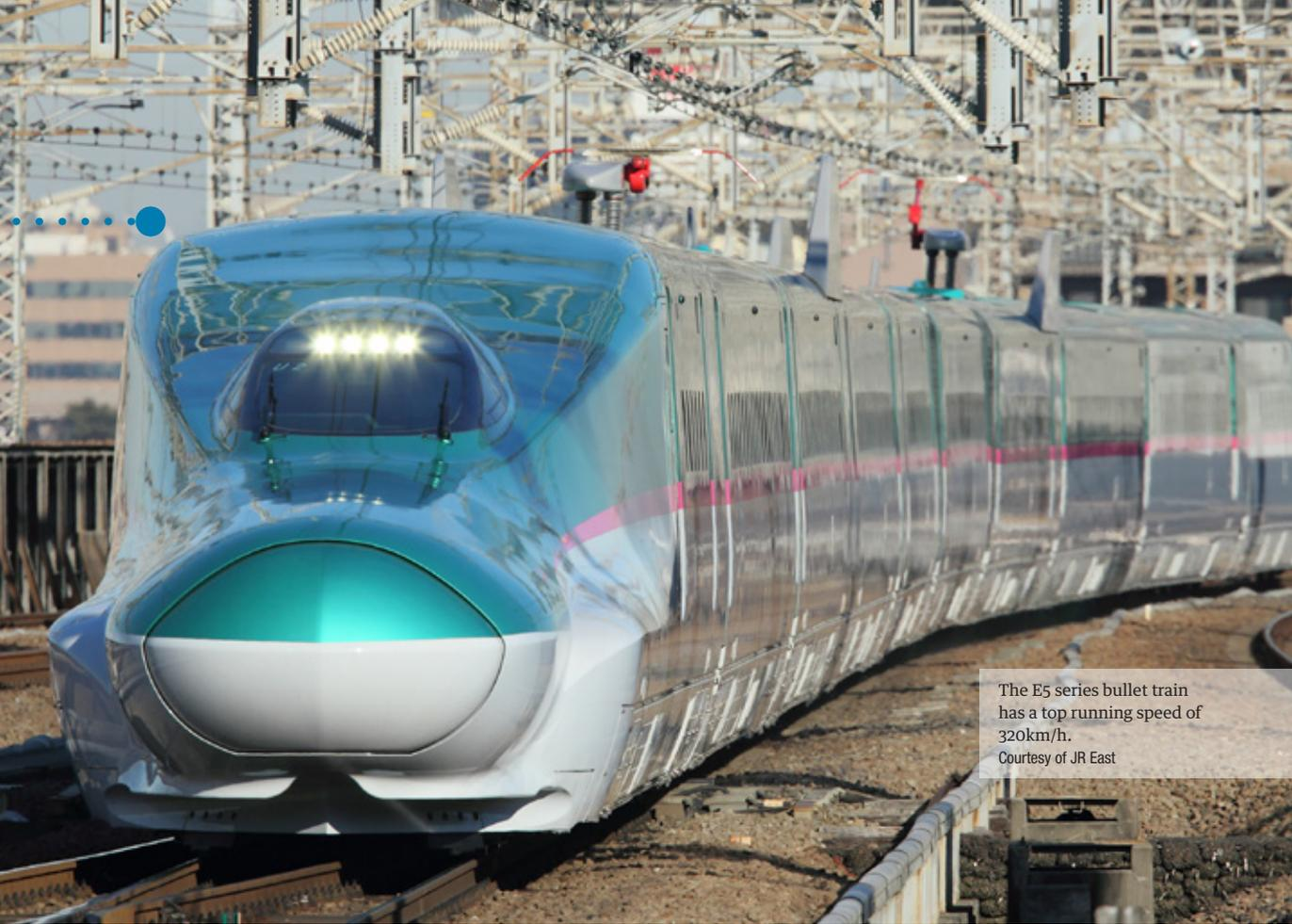
The E5 series bullet train has a top running speed of 320km/h.
