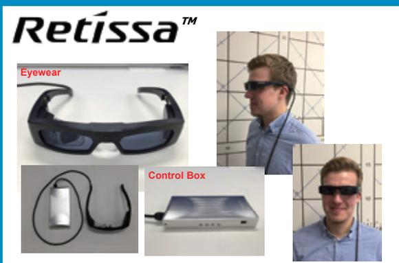
Laser eyewear (Retissa) is used by connecting a controller (300 grams) to glasses (50 grams) with a cable. Courtesy of QD Laser
