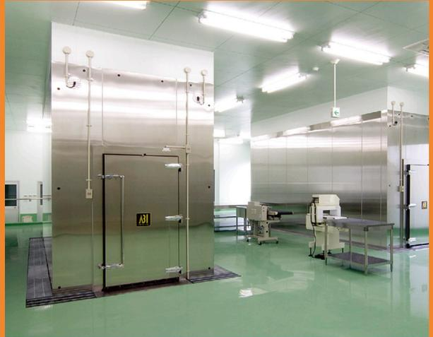
The CAS field-generating device prevents ice crystals from destroying cell walls
