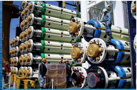
Riser pipes used in drilling
