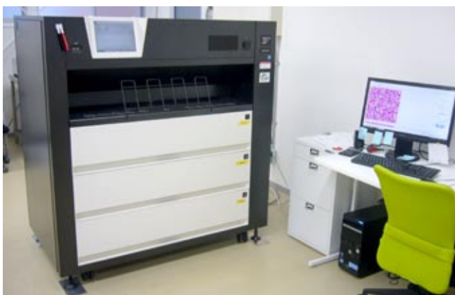
The first electrostatic textile printer, DENATEX, which employs the dye-sublimation textile-printing method. Measuring 160 cm x 85 cm x 150 cm, the printer can be positioned alongside an office desk.
