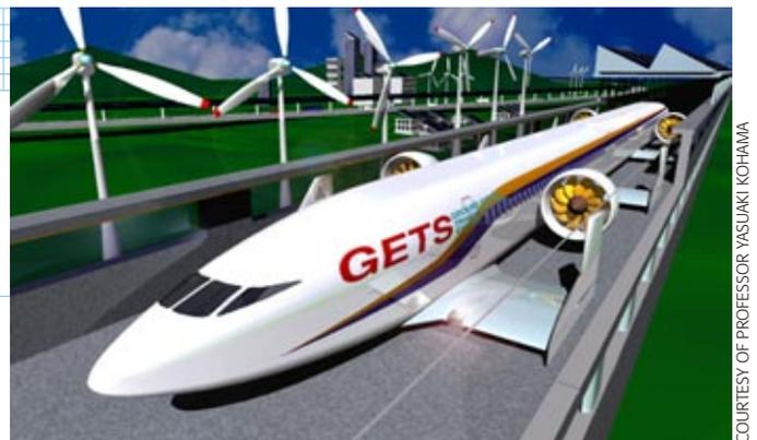
two passengers on board. The tests have produced promising results—per-unit energy consumption is less than half that of a conventional bullet train, and roughly a fifth of a linear motor (mag-lev) train. When adopted for practical use, the aim is to run the Aero-Train entirely on natural energy by covering the top portion of the guide-way with solar panels obtaining power from a special pantograph.
