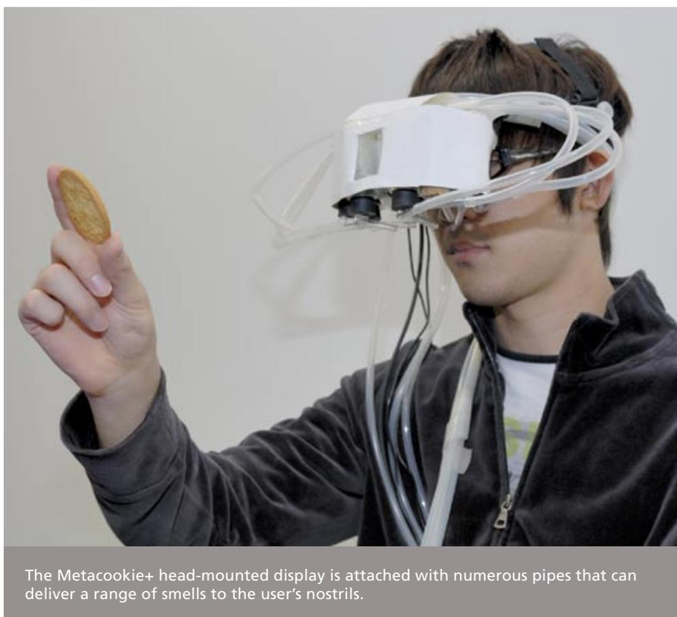
The Metacookie+ head-mounted display is attached with numerous pipes that can deliver a range of smells to the user's nostrils.
