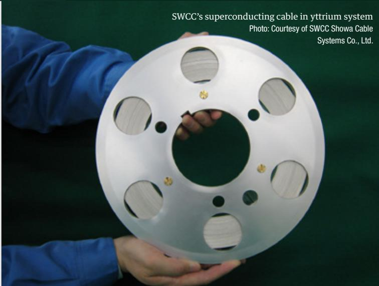
SWCC's superconducting cable in yttrium system
