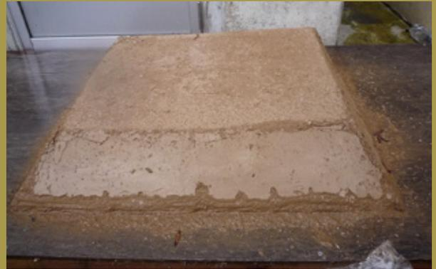
Soil solidified using general cement (left) cracks when it dries and freezes. This does not happen to soil improved using the Bon Terrain method (right).
