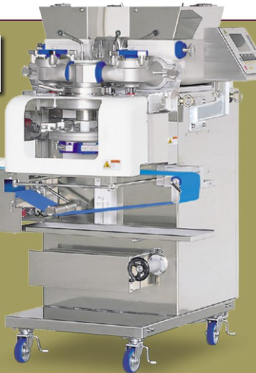
The encrusting machine manufactured by Rheon Automatic Machinery
