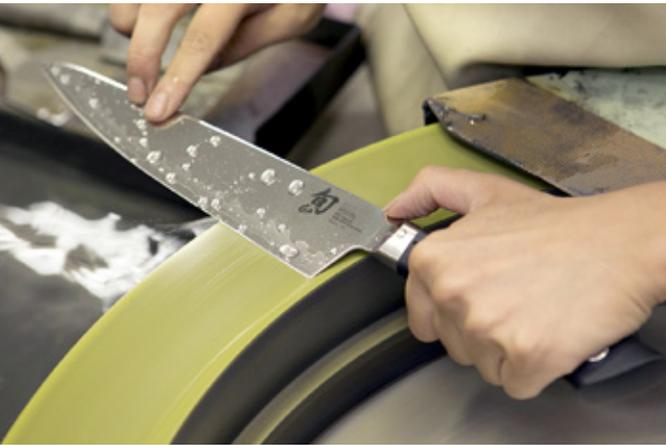
An artisan grinds and polishes a kitchen knife using a revolving donut-shaped whetstone in a process called *hatsuke*.
