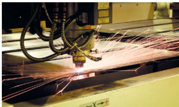
The cutting of knife blades from steel using lasers
