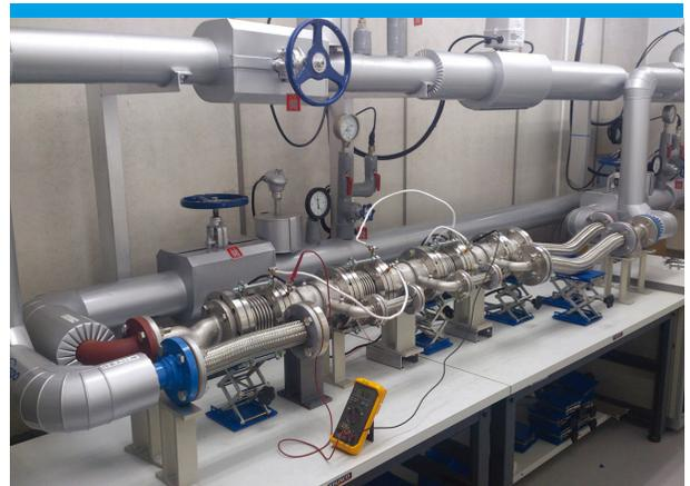
At the test facility where Yamada is using Panasonic's system to develop the thermoelectric tube for power generation
