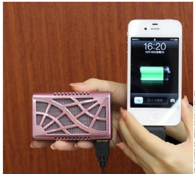
USB-compatible solid fuel type hydrogen fuel cell for recharging smartphones (left)
