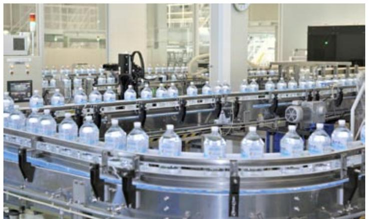
The mineral water production line at Okudaisen Bunanomori Water Plant. The snow from the snow room is used to cool the heat generated by the production line
