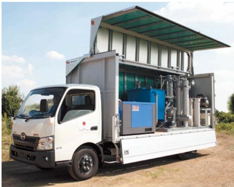
A truck fitted with the mobile ceramic membrane filtration equipment
