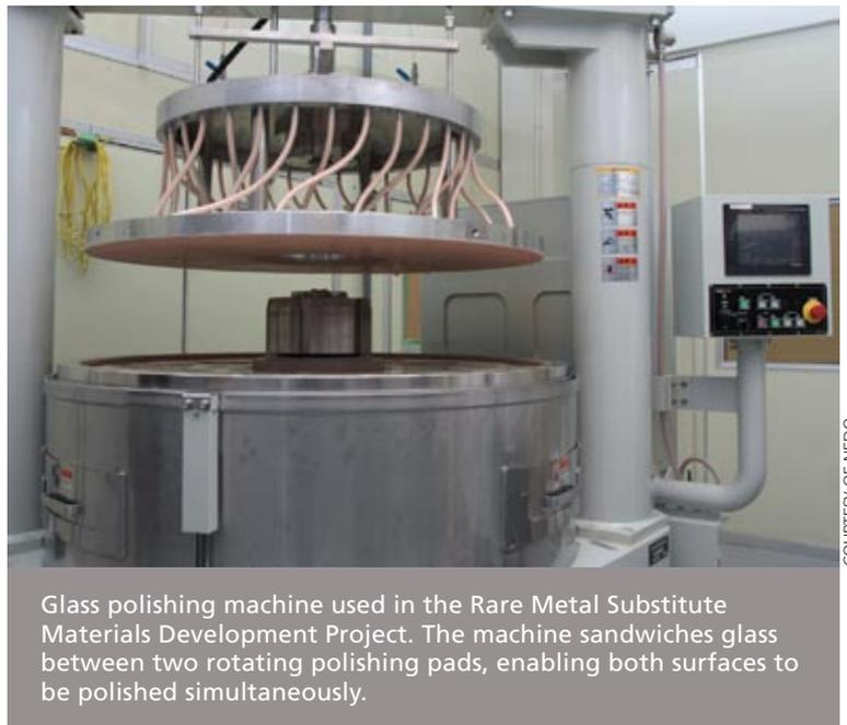
Glass polishing machine used in the Rare Metal Substitute Materials Development Project. The machine sandwiches glass between two rotating polishing pads, enabling both surfaces to be polished simultaneously.
